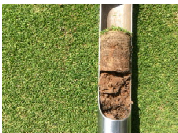
Figure 6: Very similar soil conditions were found beneath all greens. Soils were however very firm and it is important that appropriate aeration is completed going forwards including annual verti-draining. Profile beneath the 4 th green shown.
